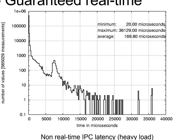
Time (average, min-max, in  $\mu$ s) **Operation** (heavy load) non real-time <u>real-time</u> 122.5, 39- 93109 75.6, 38-273 Insert Delete 18.5, 4- 41250 18.5, 8-131 22.6, 5-181681 | 25.6, 6-134 WriteData ReadData 17.0, 4- 10721 16.8, 4-62 IPC-Latency 169.8, 20- 36129 | 66.5, 21-208
